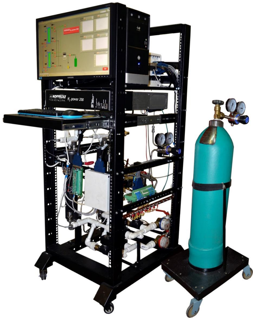
H2BioPower – 200 W (e) demonstration power unit using hydrogen +CO 2 mixture as a fuel for PEM FC
