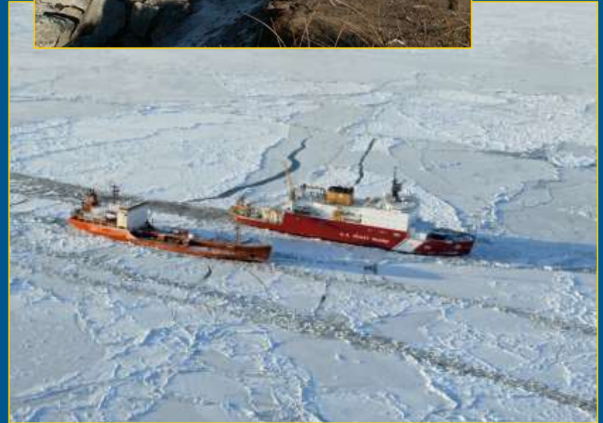
Icebreaker supported fuel delivery to Nome
